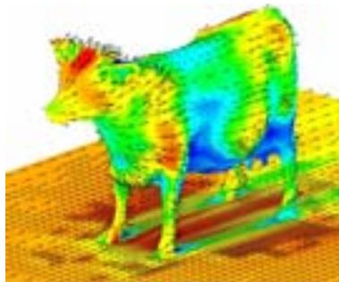
*Airflow and associated air temperature distributing around a cow in a naturally ventilated building (CFD result)*
